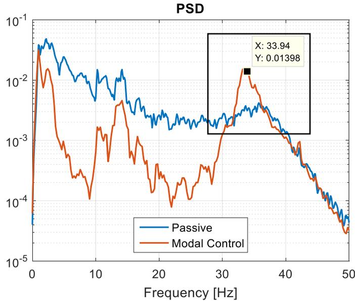
Figure 165 - Vertical modal control acceleration PSD, ideal actuator
