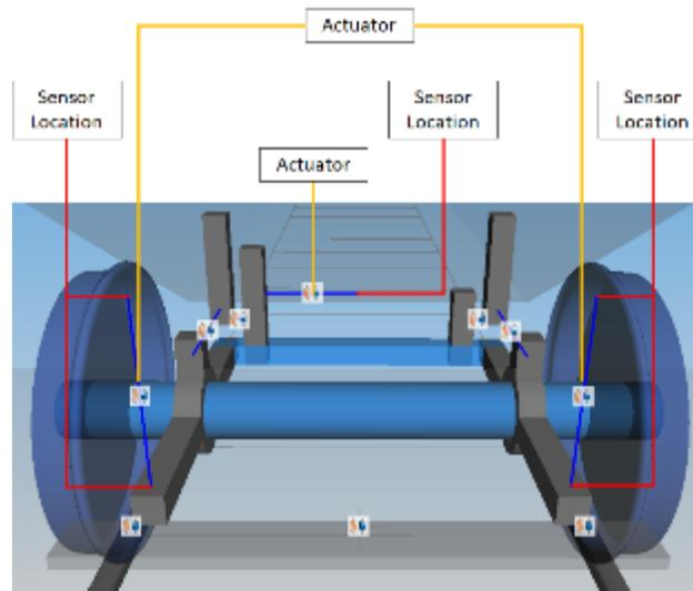
Figure 163 - Ride comfort actuators and sensors locations
