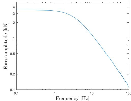
**Figure 96 - Amplitude of the fundamental harmonic of the force vs the frequency of the command variable  $\xi$**
