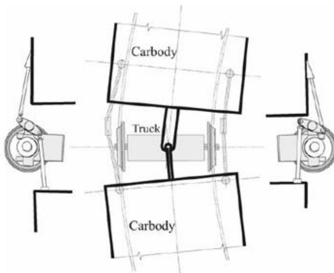
Figure 35 - Talgo's Steering Mechanism [105]
