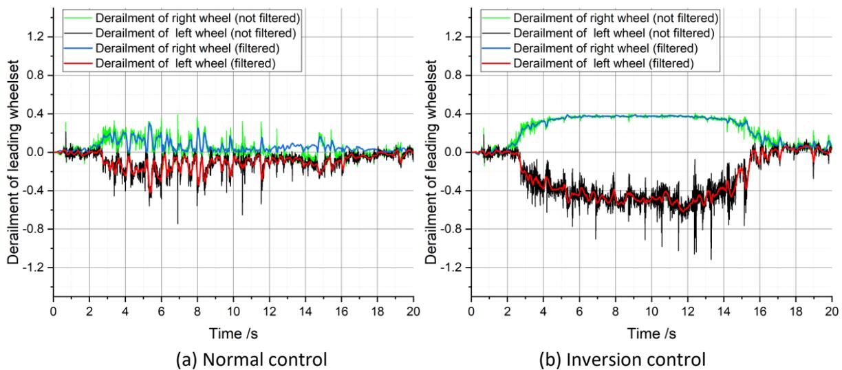
**Figure 59 - Time history of derailment coefficient (Y/Q) for scheme B2 in (a) normal control and (b) Inversion control**
