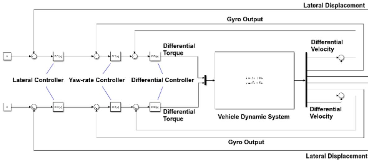
Figure 150 - Tri-loop control scheme for motorized IRW
