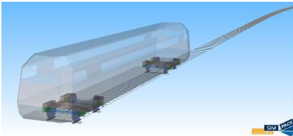
**Figure 38 - The baseline model built in Software SIMPACK**
