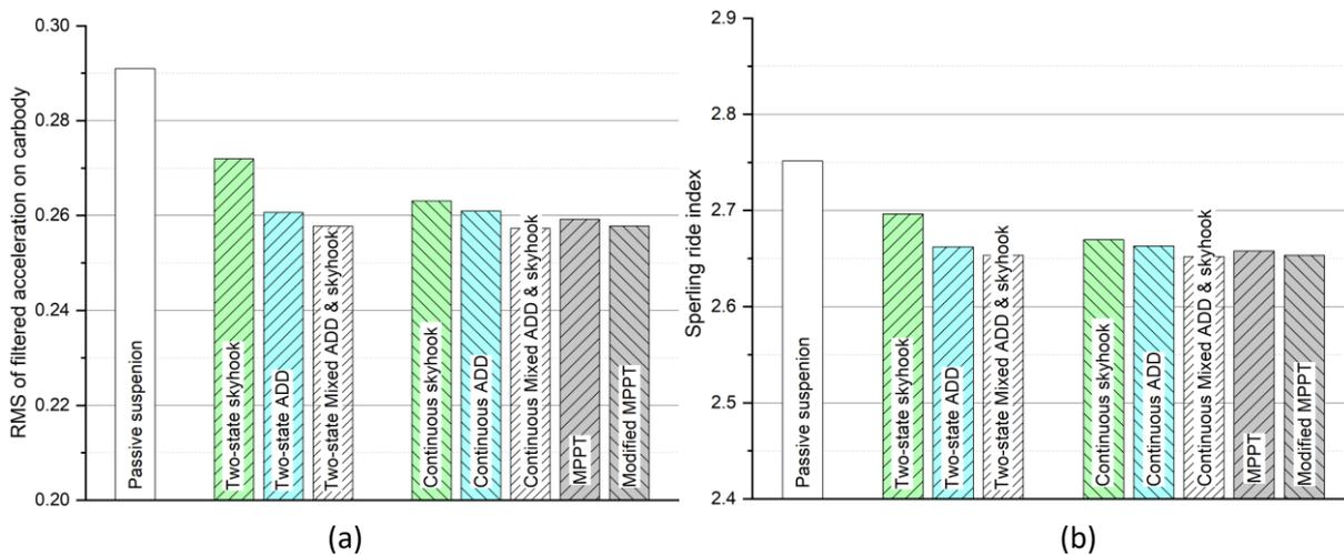
Figure 91 - Simulation results of (a)RMS value and (b)Sperling ride index with different control strategies
