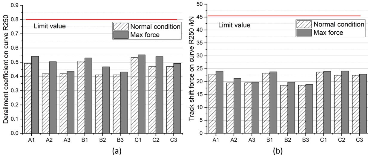
Figure 66 - (a) Derailment coefficient and (b) track shift force on R250 in normal condition and Maximum force
