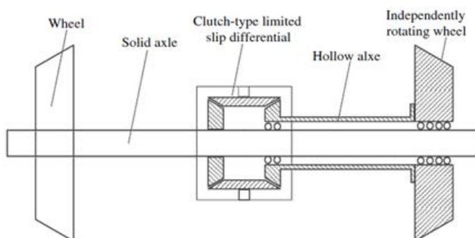
Figure 36 - Differential coupling wheelset [106]
