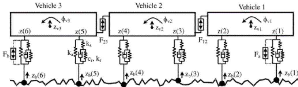
Figure 11 - Configuration for inter-vehicle actuation system [22]
