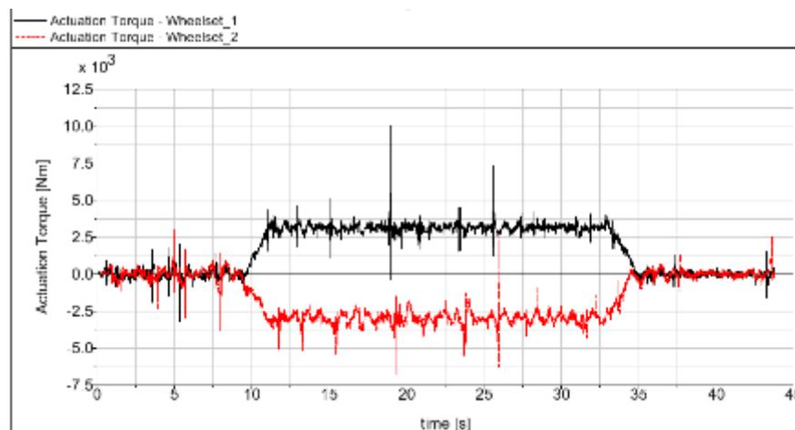
Figure 162 - Active yaw torques for dual-loop-control non-motorized IRW (with irregularities)
