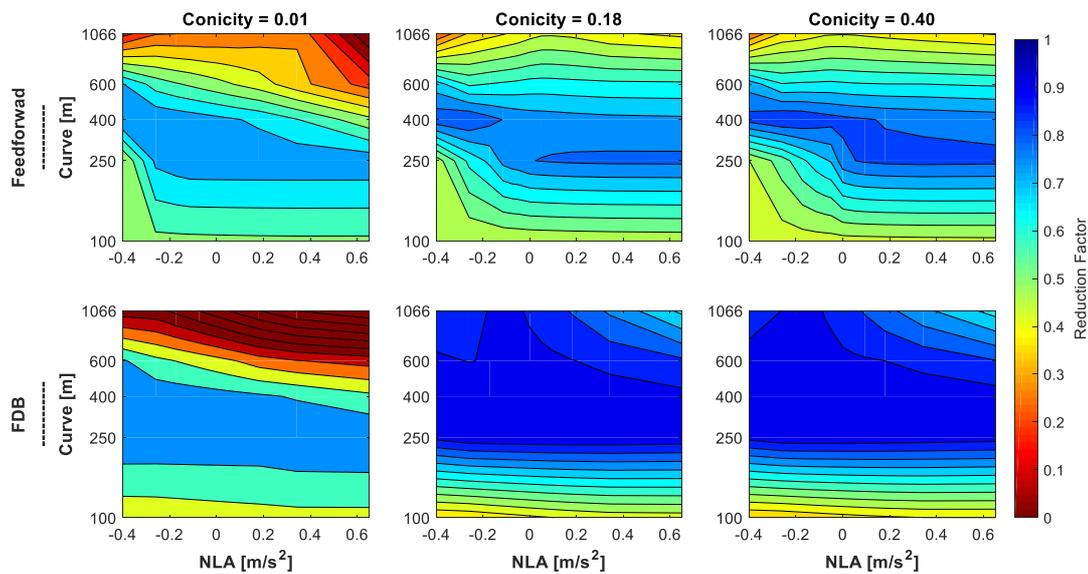
Figure 145 - Rear wheelset wear reduction distribution - HALL bush
