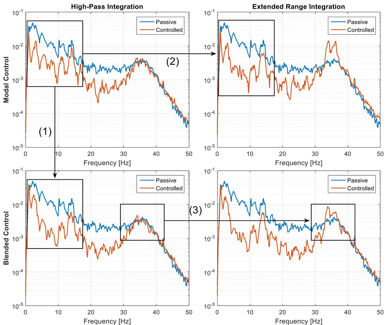
**Figure 170 - Vertical comfort control comparison**
