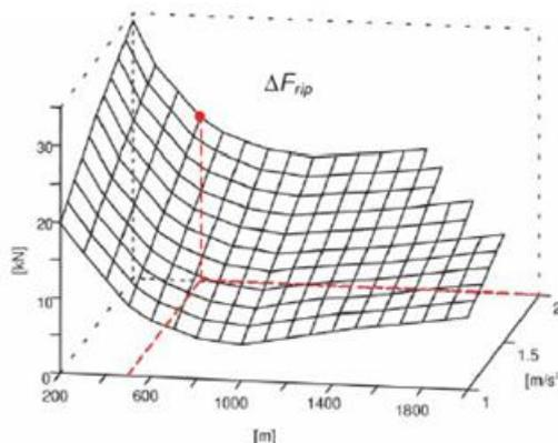
Figure 33 - Lookup table for calculating actuation force
