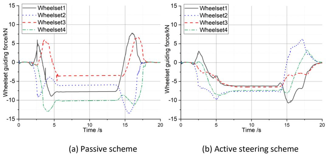
Figure 46 - Wheelset guiding force with no track irregularity
