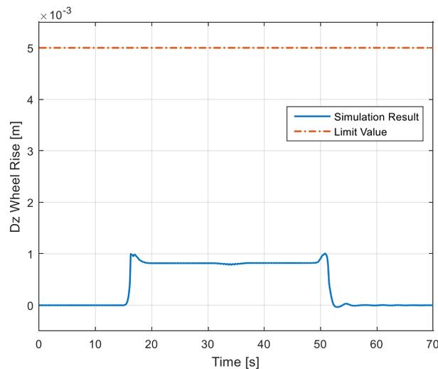
Figure 111 - Twisted track assessment EN14363 [128] - method 1
