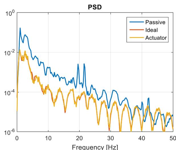
**Figure 171 - Real vs Ideal actuator lateral decentralized control acceleration PSD**
