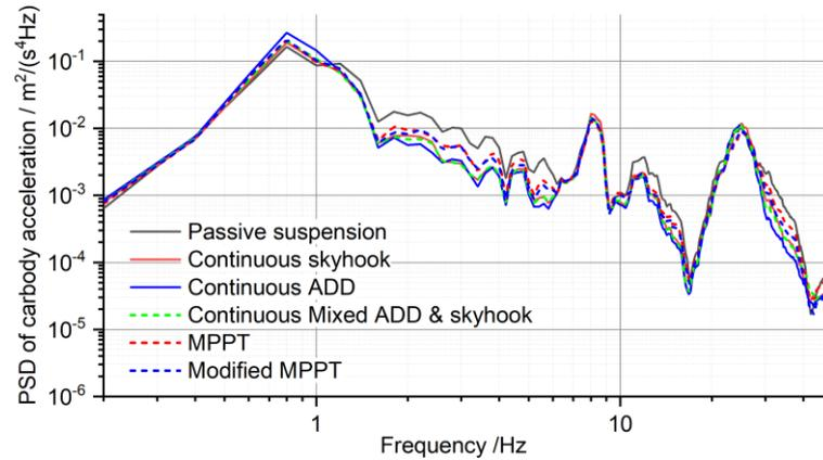
Figure 90 - PSD analysis on the effects of continuous control strategies
