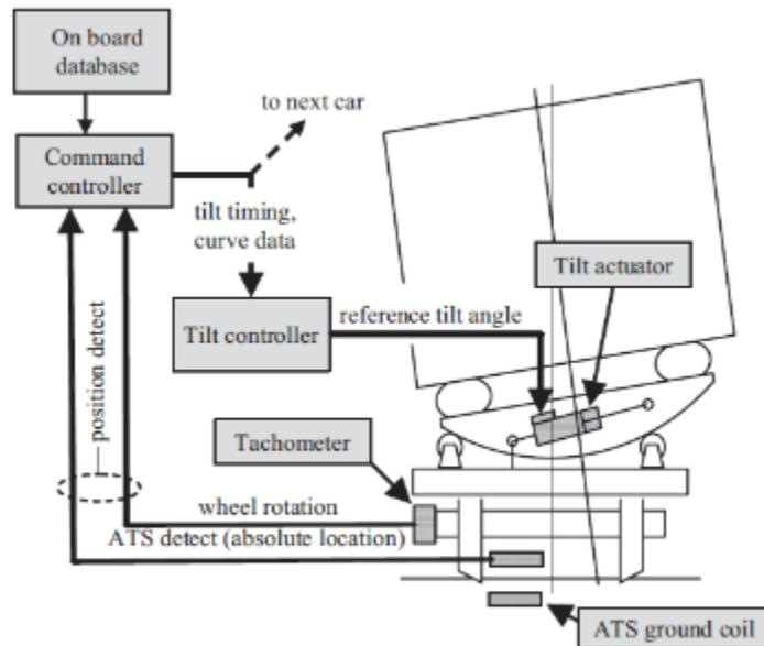
Figure 5 - Controlled Natural Tilting [6]
