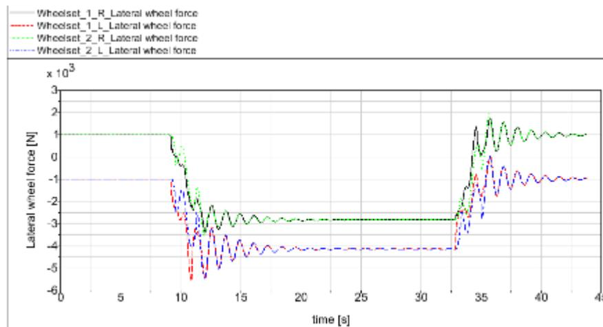
Figure 159 - Wheel/rail lateral forces for dual-loop-control non-motorized IRW (without track irregularities)
