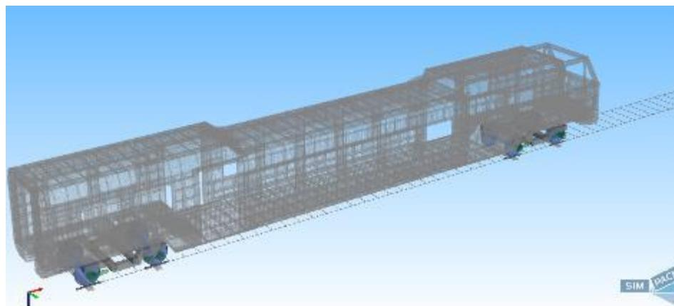
Figure 73 - Full vehicle model considering car body flexibility
