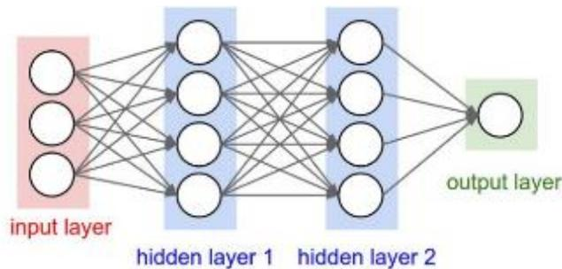
Figure 77 - The layers of the Neural Network
