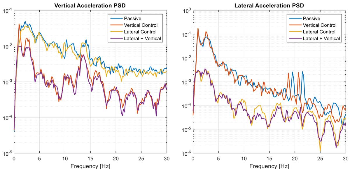
**Figure 176 - Vertical and Lateral comfort control comparison: vertical acceleration PSD (left), lateral acceleration PSD (right)**
