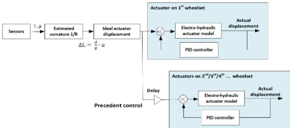
Figure 44 - Workflow of first active steering control
