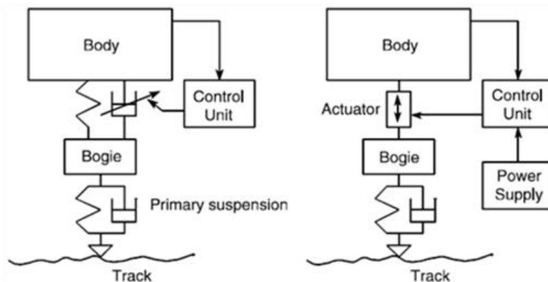
Figure 2 - Schematic diagram for the principles of semi-active (left) and fully-active (right) suspensions
