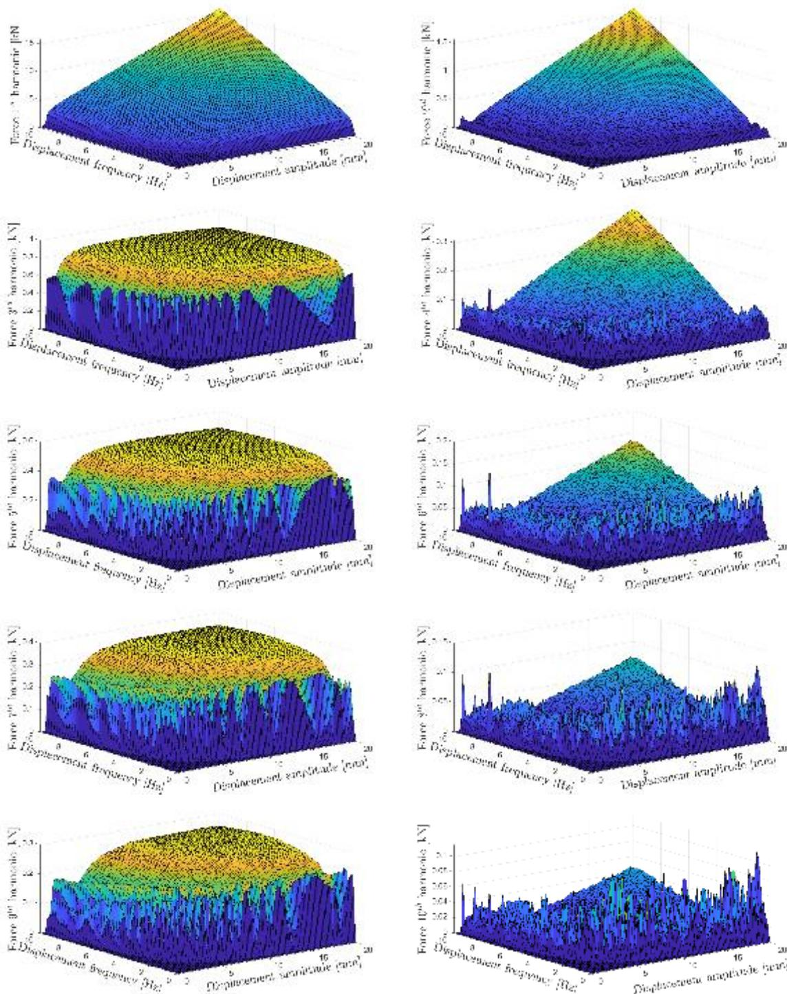
Figure 100 - Amplitude of the harmonics 1 to 10<sup>th</sup> associated with the actuator force when a harmonic displacement in the rod is applied
