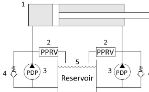
Figure 93 – Actuator hydraulic scheme
