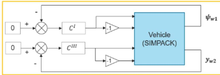
Figure 119 - Combined steering control scheme
