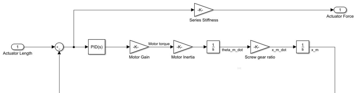
Figure 132 - Electromechanical actuation model
