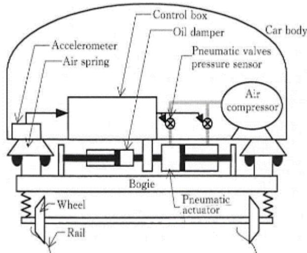
Figure 20 - Prototype of Series 500 EC [70]
