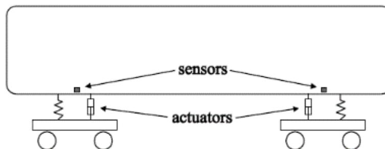
Figure 9 - Active Secondary Suspension System [21]
