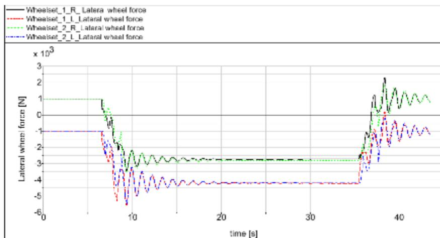
Figure 134 - Wheel/rail lateral forces for yaw relaxation control (without track irregularities)
