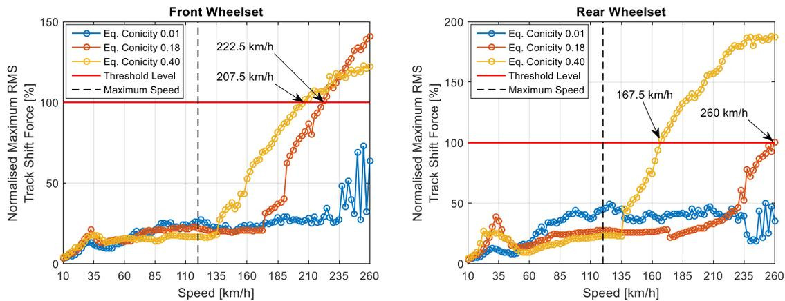
Figure 140 - HALL stability assessment - Track shift force front (left) and rear (right) wheelset
