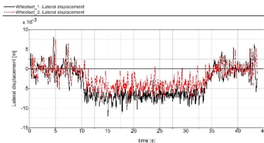
Figure 151 - Wheelset lateral displacement for dual-loop-control motorized IRW (with track irregularities)
