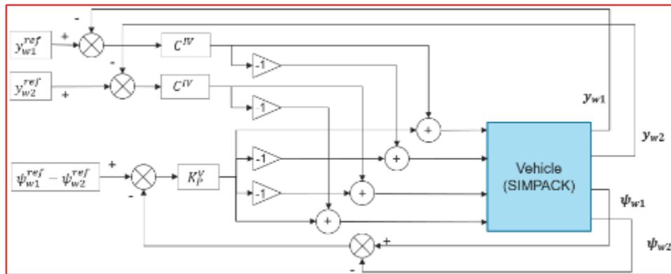
Figure 120 - Creepage steering control scheme
