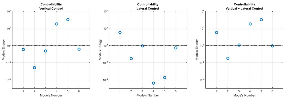
**Figure 174 - Modes controllability for different control approach: Vertical control (left), Lateral control (center) and Vertical plus Lateral control (right)**
