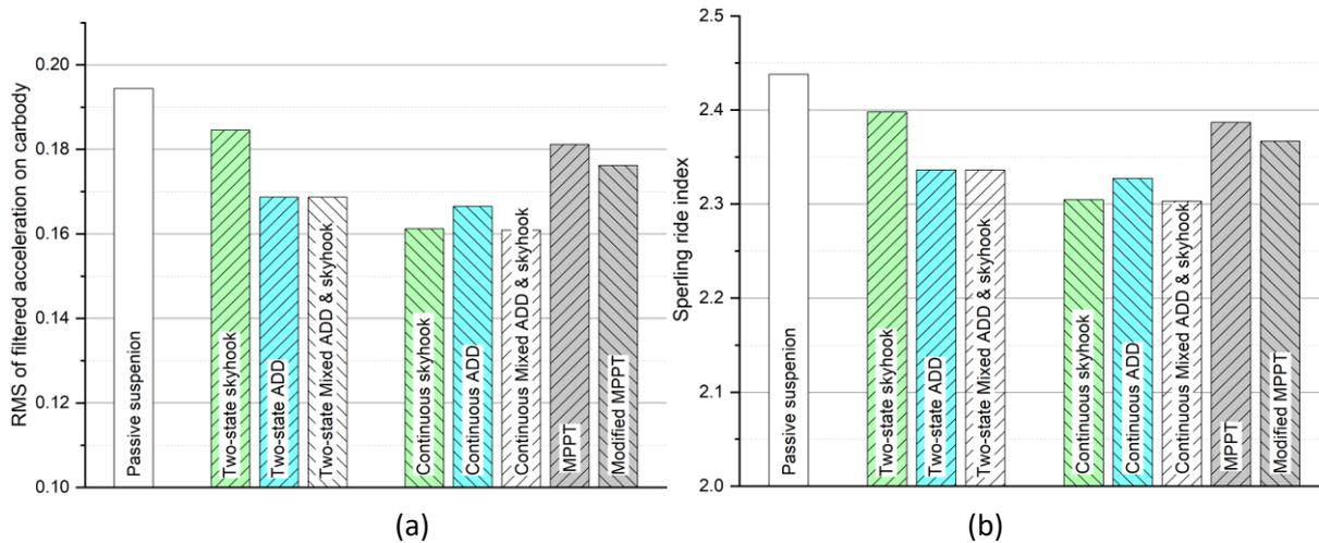
Figure 88 - Simulation results of (a)RMS value and (b)Sperling ride index with different control strategies
