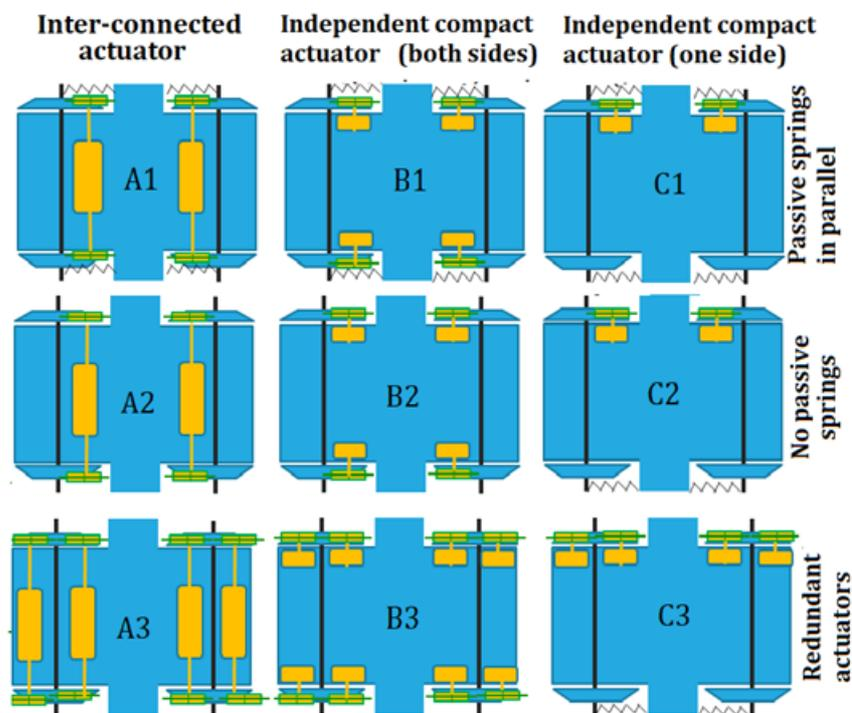
Figure 55 - The “three by three” active steering schemes
