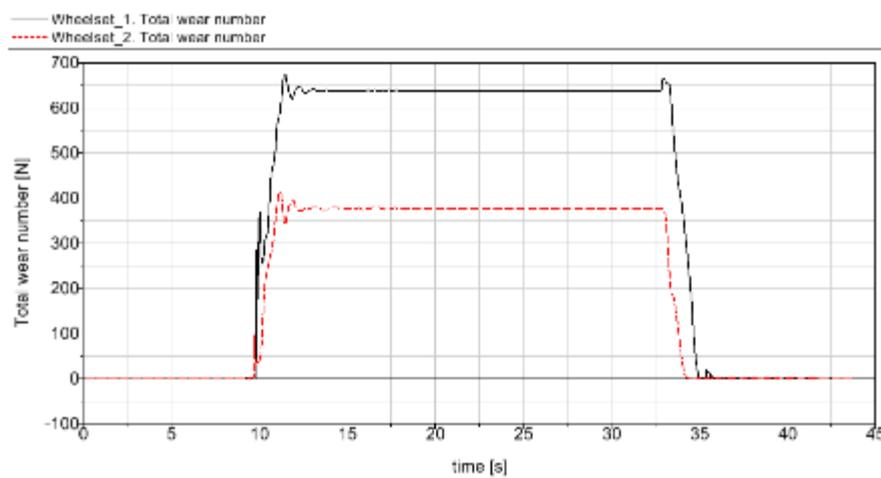
**Figure 148 - Wheelset total wears for passive IRW vehicle (without track irregularities)**
