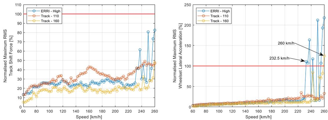
Figure 115 - Stability assessment, case b): track shift force (left), wheelset acceleration (right)
