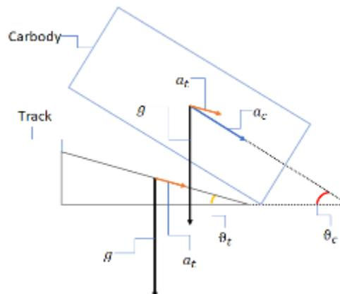
**Figure 110 - Sway model calculation**
