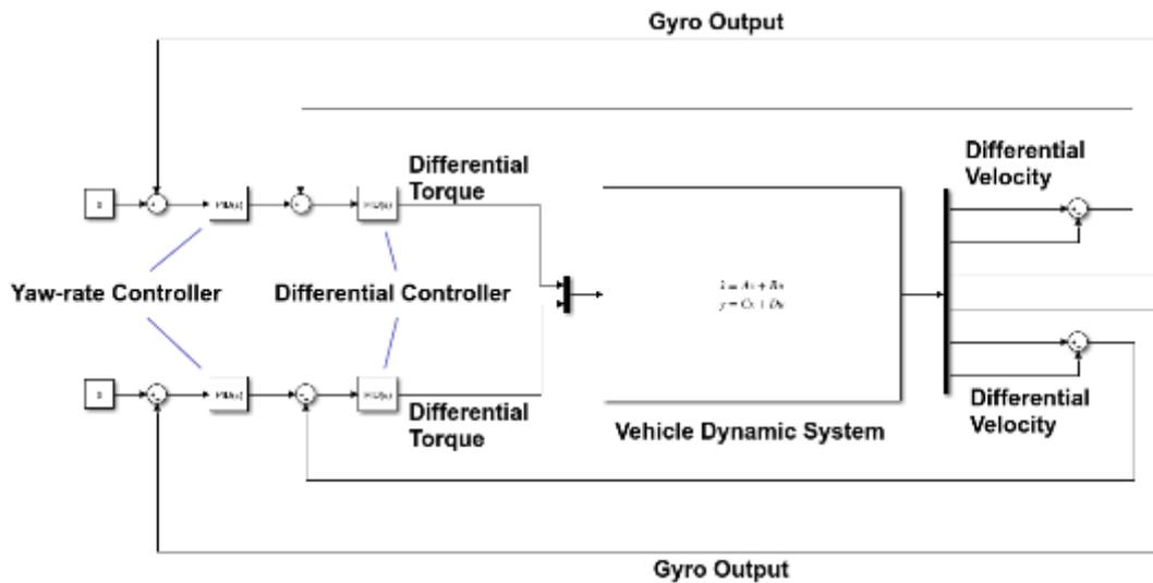
Figure 149 - Dual-loop control scheme for motorized IRW
