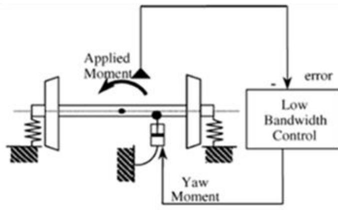
Figure 32 - Control strategy based on yaw moment applied from primary suspension
