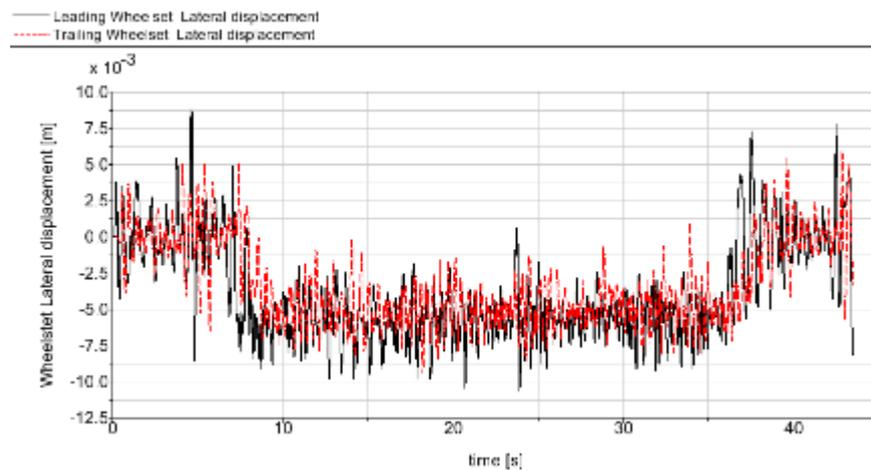
Figure 133 - Wheelset lateral displacements for yaw relaxation control (with track irregularities)
