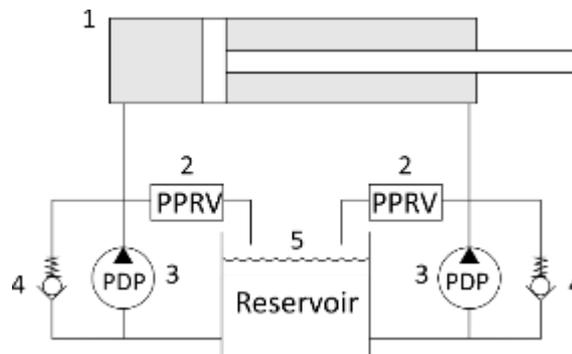
**Figure 167 - Double acting hydraulic actuator**
