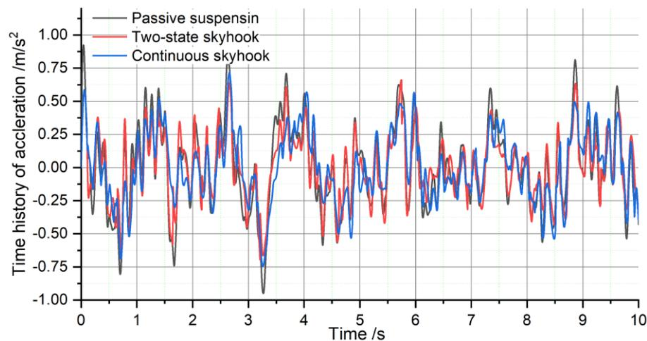
**Figure 82 - The time history of acceleration with different suspension systems**
