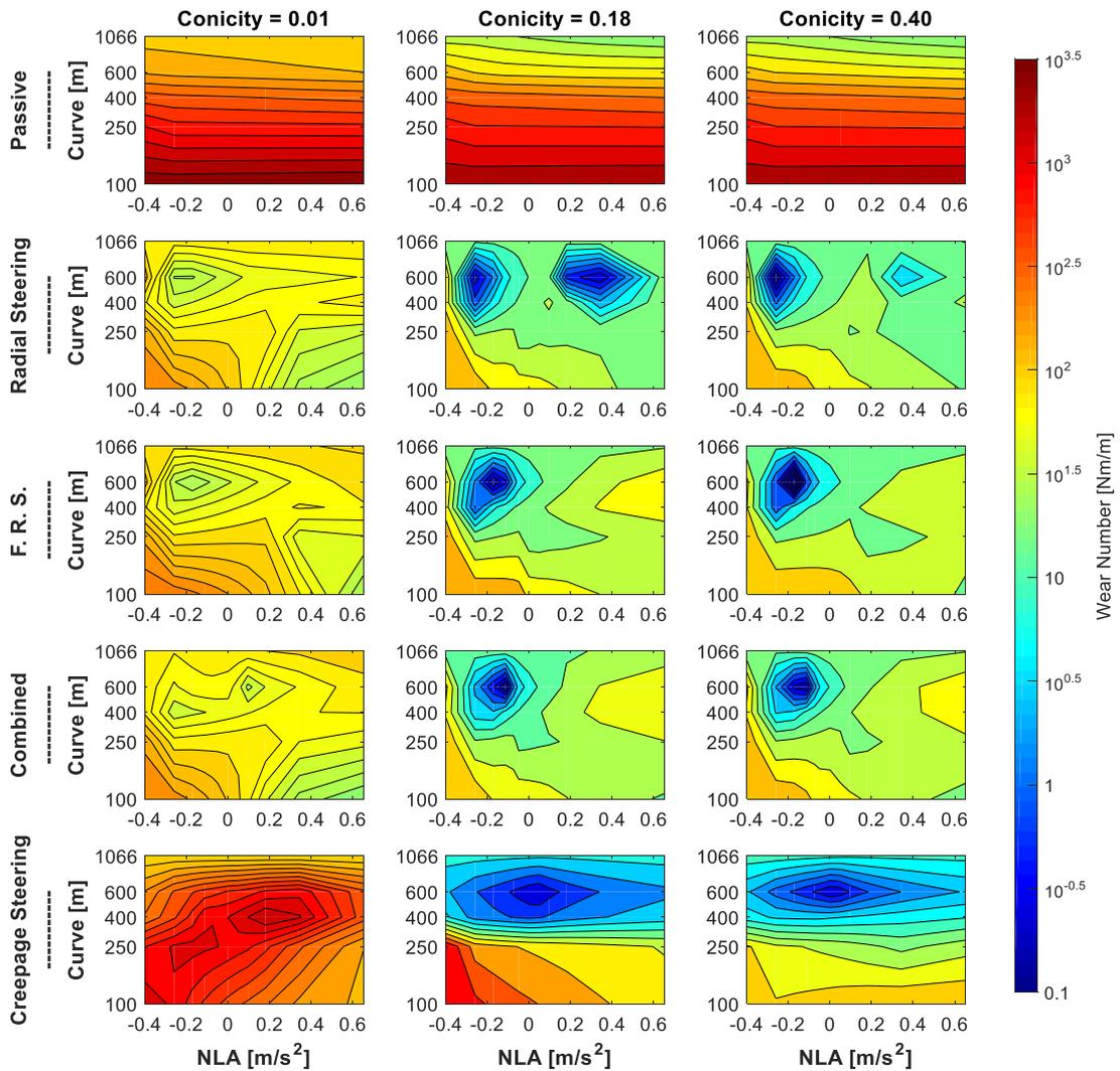
Figure 121 - Front wheelset wear distribution - Feedback approach
