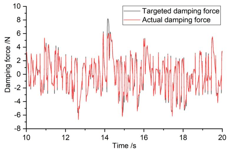
**Figure 79 - Comparison between the targeted damping force and actual damping force**
