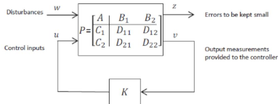
Figure 15 -  $H_\infty$  Control Scheme
