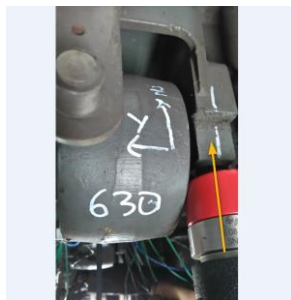
Figure 93: Driving point on the bogie
