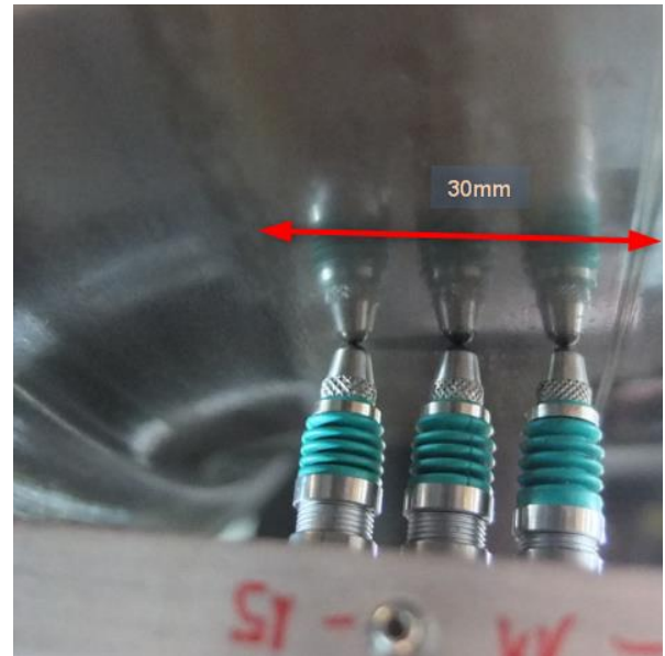
Figure 75: Contact area of Wheel 4 with displacement sensors
