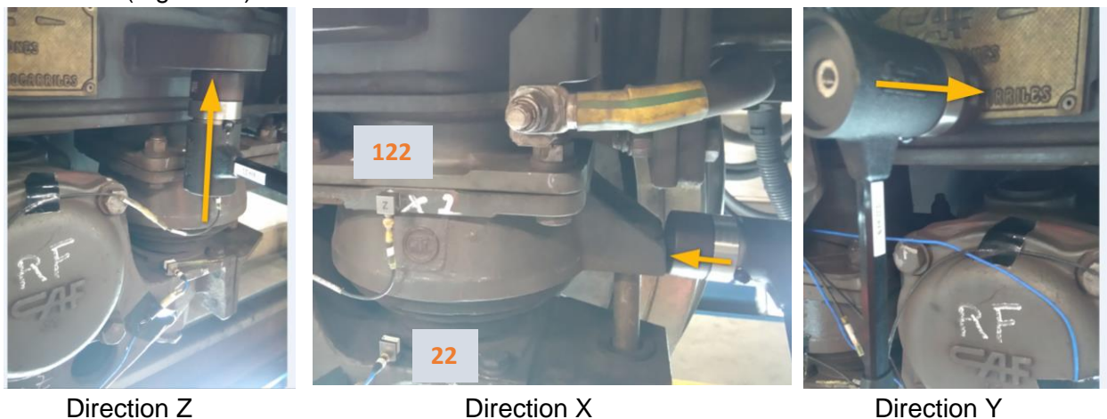
Figure 85: Driving point location bogie (122) – response location 22 is on the wheel set side (upstream)
